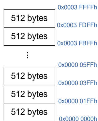
SC32L14T 256 Kbytes Flash ROM Sector Partition Illustration
